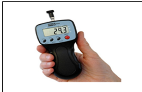
Figure 3.11: Pressure Pain Simulation System *Wagner FDX-25 device (Wagner Instruments, Greenwich, CT)
